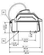
Electrical inlet (power) Electrical Outlet
